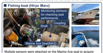
the data necessary to check the seal performance in multiple driving
